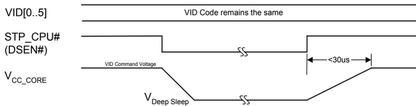
**FIGURE 6. Vcore RESPONSE FOR DEEPER SLEEP COMMAND**
