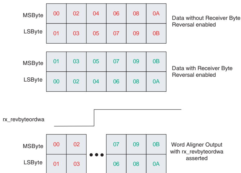
Figure 1-57. Receiver Byte Reversal Feature
