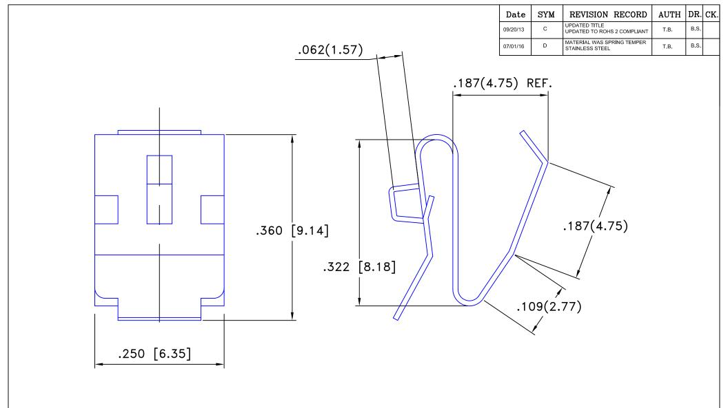
MATERIAL: 0.010" SPRING STEEL, NICKEL PLATED ROHS 2 COMPLIANT
