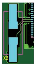
Figure 2 Sample 20 MHz Crystal Routing
