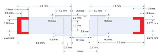
Figure 3 Triple 20 MHz crystal footprint with solder mask over pad
