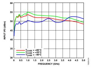
Figure 14. Input IP3 vs. Frequency over Temperature,  $V_{\rm DD} = 5~{\rm V}$
