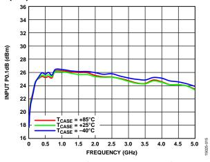
Figure 15. Input 0.1 dB Power Compression (P0.1dB) vs. Frequency over Temperature,  $V_{DD} = 3 V$
