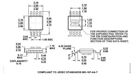
Figure 19. 8-Lead Mini Small Outline Package with Exposed Pad [MINI\_SO\_EP] (RH-8-3) Dimensions shown in millimeters
