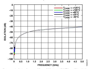
Figure 11. Isolation Between RF1 and RF2 in an All Off State (EN =  $V_{DD}$ ) vs. Frequency over Temperature
