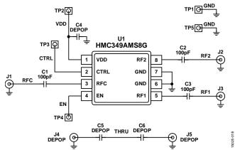
Figure 19. Evaluation Board Schematic
