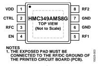
Figure 3. Pin Configuration (Top View)
