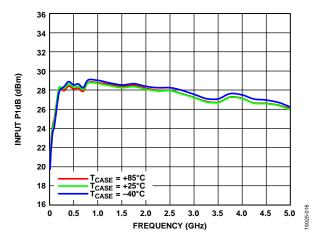
Figure 16. Input 1 dB Power Compression (P1dB) vs. Frequency over Temperature,  $V_{DD} = 3 V$
