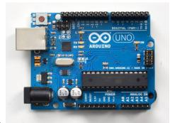
Begin by breaking the 36-pin male header into four pieces: one 10-pin, two 8-pin and one 6-pin. Stick the header into the Arduino sockets with the long pins down.
