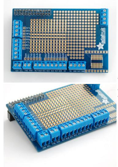
Place the blue terminal blocks around the perimeter of the Proto Plate PCB. Make sure you place them so that the open ends are facing out as shown.
