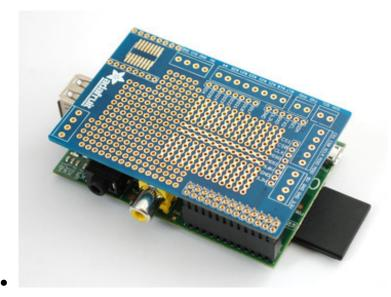
Place the proto plate PCB on so that the 2x13 header pins poke out through the matching 2x13 pads in the corner.
