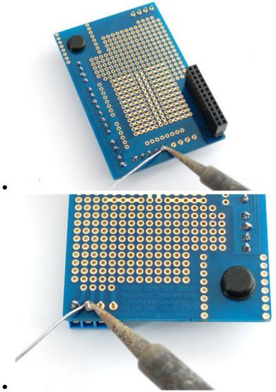
Solder each terminal block connection to the PCB using plenty of solder to make a strong mechanical connection
