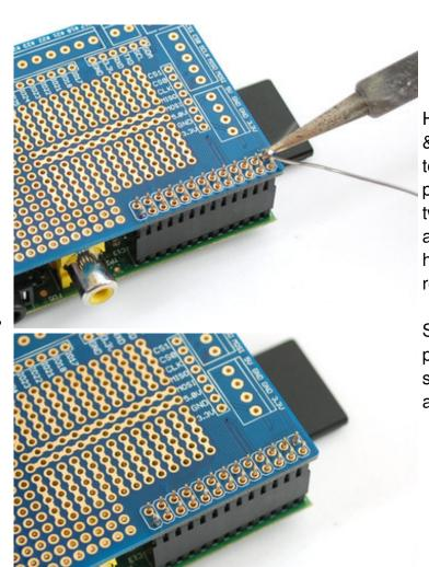
Heat up the soldering iron to 650 °F and wait for it to get up to temperature. Then heat a corner pad/pin with the iron tip and after two seconds poke in a small amount of solder. After the solder has melted into the pad/pin remove the iron.
