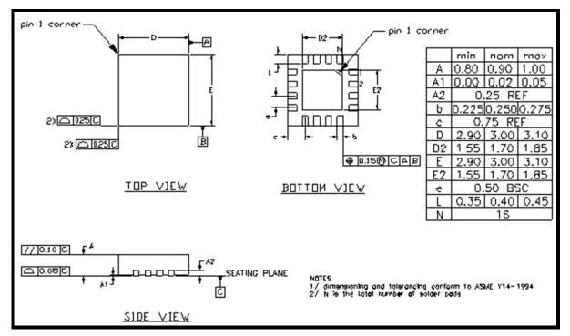
Figure 4: SE2537L Package Diagram
