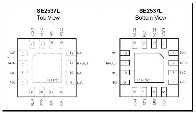
Figure 2: SE2537L Pin-Out Diagram
