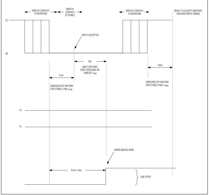
Figure 4b. Wiper Transition Timing Diagram—Timed Out
