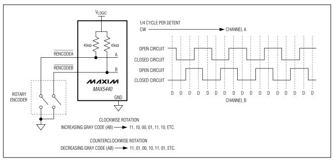
Figure 1. Rotary Encoder Interface
