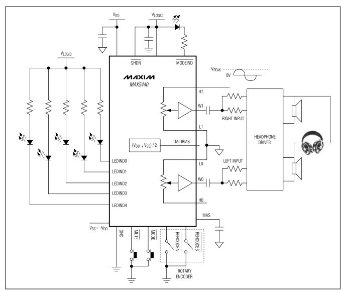
Figure 6. Dual-Supply Volume/Balance Control
